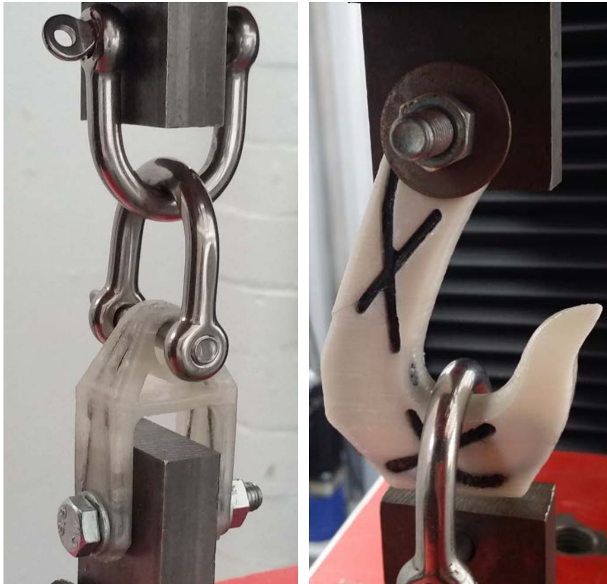
Figure 8. Fixtures for pulley and hook tests.
