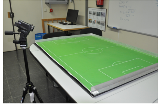
Fig. 8 Video camera mounted on a tripod and scale soccer court model.
