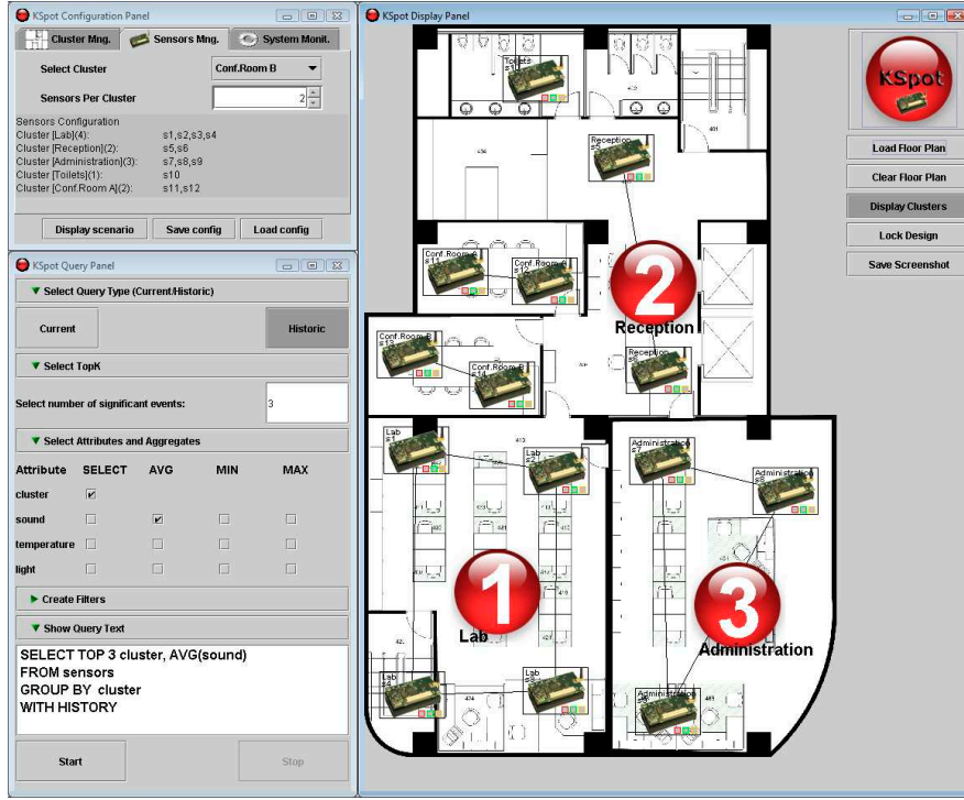
Fig. 3 KSpot's Graphical User Interface (GUI) allows users to administer the execution of Top-K Queries through an intuitive and declarative user interface. The above scenario conducts a Top-3 query over a 14-node sensor network organized in 6 clusters. The Display Panel (on the right) illustrates the three KSpot-Bullets for the three highest-ranked sensor clusters.
