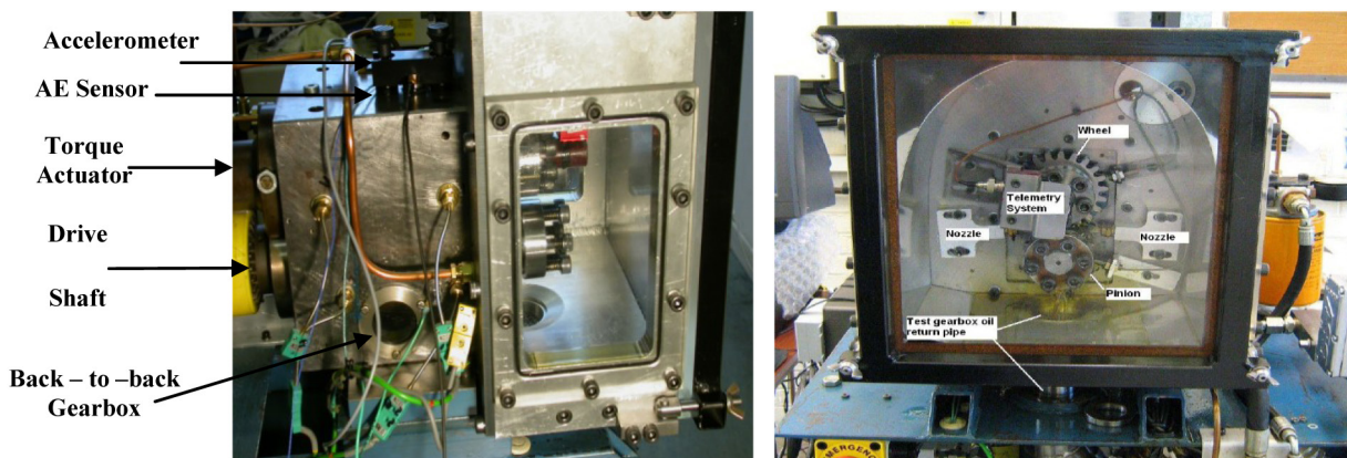
Figure 1. Newcastle University 75 mm centre distance back-to-back gear test rig
