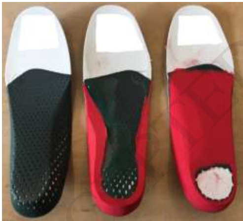
Fig. 1 Stages of insoles being supported with shore 30 EVA
