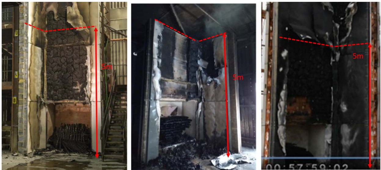
Figure 13 PIR/A2 comparison of burn area DCLG (left), FPA (centre) and Čolić (right) [17, 19]
