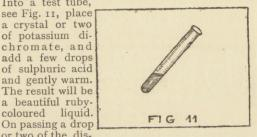
or two of the distillate into the tube, if any alcohol is present the whole will be changed, on gently agitating it, from ruby to green. This is a chemical test, and gives us further proof that alcohol is present.
