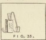
with water, and a piece of bent glass tubing or india-rubber tubing is placed in it, as shown. On drawing all the air out of the tube with the mouth the water begins to flow, and will
