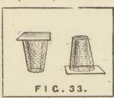
physical properties, and some interesting experiments may be shown. Fill a tumbler completely full of water, as shown in Fig. 33, and cover it with half a sheet of stiff paper. The glass may then
