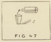
acid gas, and pour it, as shown in Fig. 47, into the tumbler. The heavy carbonic acid gas will fall into the tumbler and diplace the lighter air. After a minute or so remove the jar and plunge the lighted taper into the tumbler; it will at once be extinguished. Pour a little lime water into the tumbler, it will at once become turbid. The experiment proves that the carbonic acid gas must be heavier than air.
