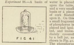
upon the table, and a very small basin or a piece of cork floated upon it. On this a small fragment of phosphorus is placed and ignited, and immediately covered by a bell jar, as shown in Fig. 41. The phosphorus
