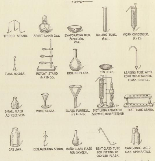
THE above sketches show the whole of the apparatus for the 76 experiments to be shown in the 12 articles in this magazine during 1896 on the following subjects:
