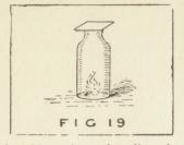
mouth of the bottle with a piece of cardboard, and the flame will be extinguished; by the aid of a piece of wire remove the sponge, and add to the bottle a little clear lime water and well shake. The lime water will become turbid owing to the
