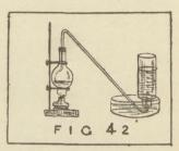
applied by means of spirit lamp. The oxygen is given off and displaces the water. should be collected, and corked ready for use, or they can be stood mouth downwards in saucers full of water.
