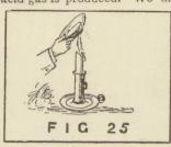
certain that the fat is rich in carbon. If, when the candle is alight, we hold a cold saucer in the flame, as shown in Fig. 25, we shall obtain upon the saucer a thick deposit of carbon, all of which,
