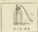
the bottle place some fragments of marble. Then pour down the funnel some dilute hydrochloric acid. Marble is calcium carbonate, and as soon as the acid comes into contact with this it forms
