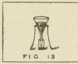
port wine and well shake. The whole mass is blackened, now pour upon a funnel fitted with a filter paper as shown in Fig. 13. The wine will filter through perfectly clear, the colouring
