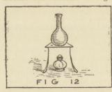
the gas escapes the alcohol re-mains behind in the liquid. Let us take a sample of brewer's the handiwork - a little ale, and put it in a flask and heat it as shown in Fig. 12. Just as the liquid boils
