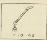
muslin, mix it with a little soda lime, transfer it to a test tube and heat over a spirit lamp; fumes will quickly be given off smelling something like burnt feathers. Moisten a piece of red litmus paper and hold
