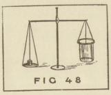
in a much more striking and positive way by means of a fairly delicate pair of scales. Remove one of the pans attach a and glass beaker, as shown in Fig. 48, exactly counterpoise with weights. Now
