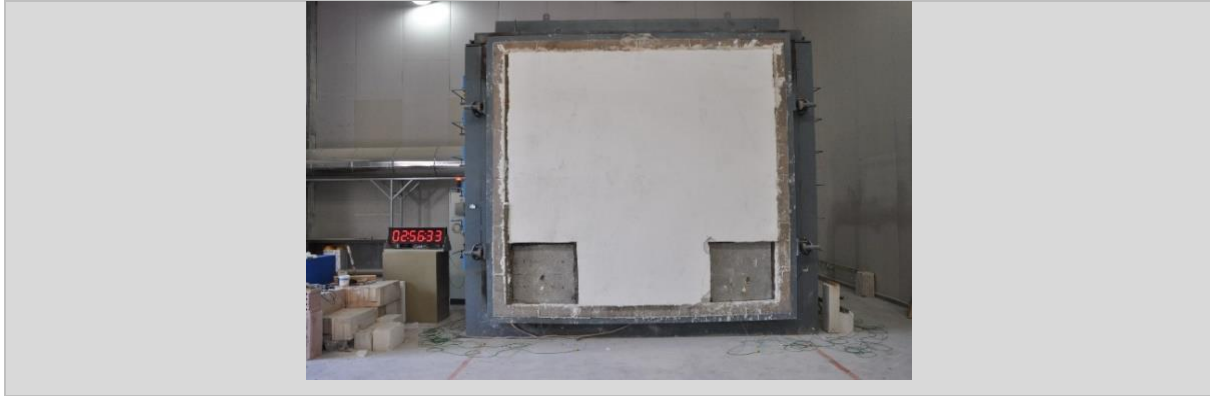
Figure 11. Experimental configuration of the embedded specimens in a walled metal steel frame in the large-scale furnace (specimen of interest: the one on the left).
