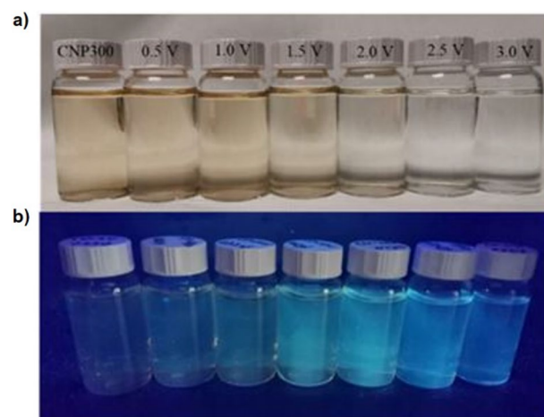
Figure 3. Photos of 0.02 \text{ mg ml}^{-1} C-dots dispersions in 0.15 \text{ M KCl} that has been subjected to chronoamperometry treatments for 60 s at applied voltages from 0.5 to 3.0 V compared to the untreated sample under (a) daylight and (b) UV-radiation.
