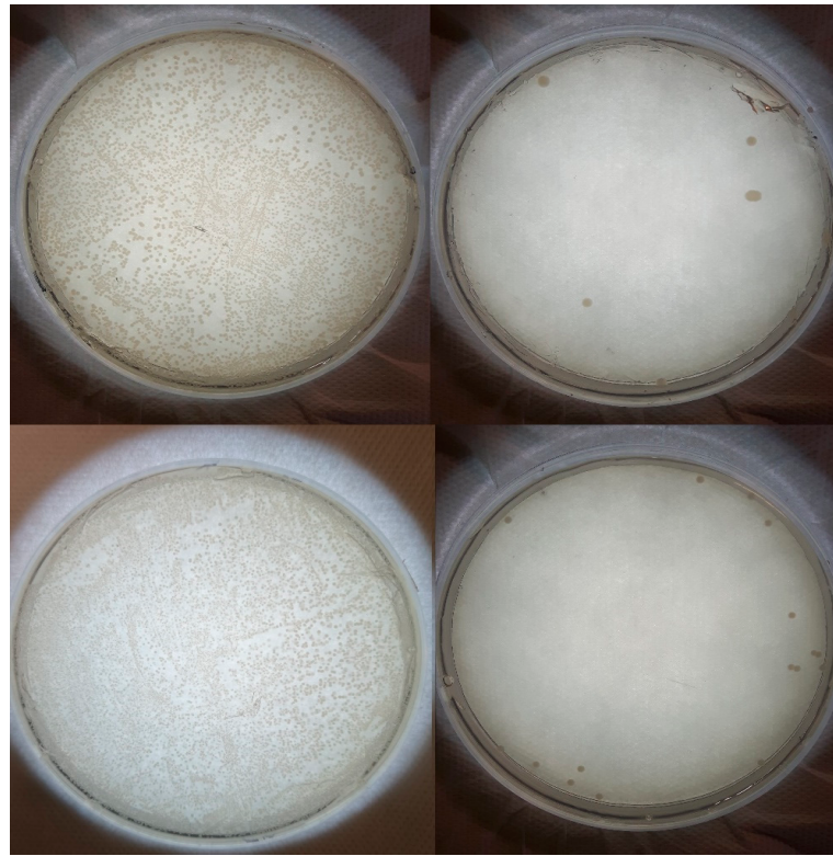
Figure 3. Agar spread plates of E. coli (top) and S. aureus (bottom). The leftmost photos were cultured on uncoated QCM-D crystals, while the rightmost photos were cultured on (Naf/CDot) 6 -coated discs. Each control–test pair was taken at the same dilution.
