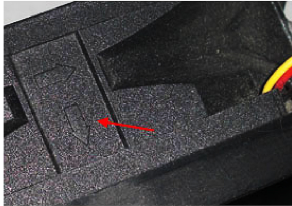
Fig. 6. Signs on ventilator specify fan blades rotation and airflow direction [7].
