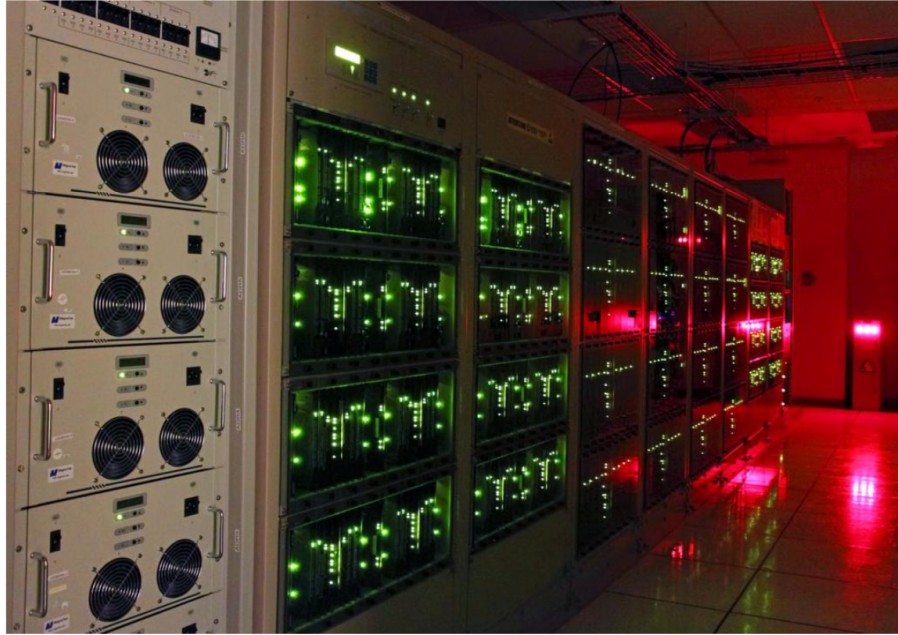
Figure 2.7: The ALMA 64-input Correlator used by the 12-m array. This is located in the ALMA Array Operations Site Technical Building. Image credit : ALMA (ESO/NAOJ/NRAO), S. Argandoña.
