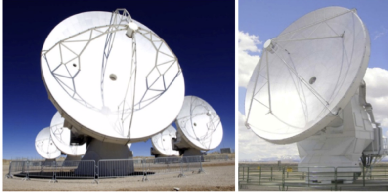
Figure 2.3: The two types of antennae used in the 12-m array. Right shows the VertexRSI antenna whilst left is the AEM antenna. Image adapted from Remijan et al. (2020).
