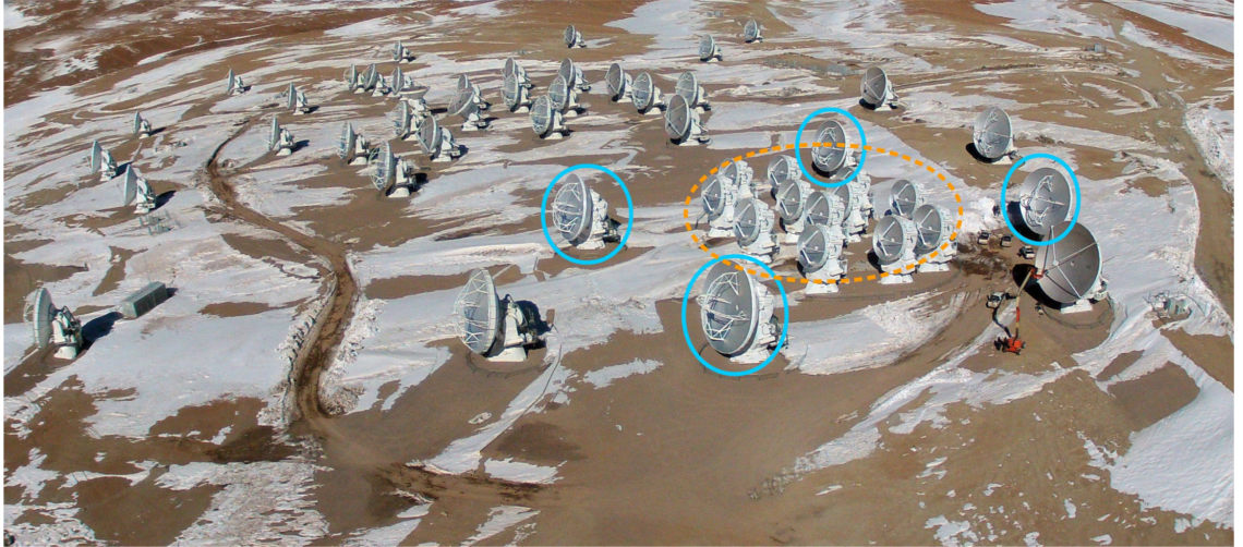
Figure 2.2: The ALMA interferometer, located on the Chajnantor plain of the Chilean Andes. The 50 antennae in the 12-m array are located on the left and are un-circled. The 12 7-m dishes in the ALMA Compact Array (within the orange dashed circle) and four single-dish 12-m dishes (blue circles) can be seen on the right (Remijan et al. 2020).
