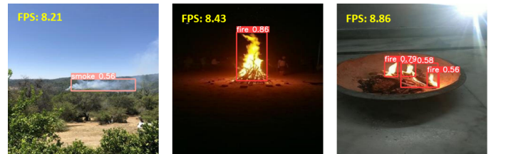
Fig. 6. Evaluation on the Raspberry Pi platform: the detection result of the image obtained in real time from the web camera, with the live detection frame rate in the top left corner of the detection screen.
