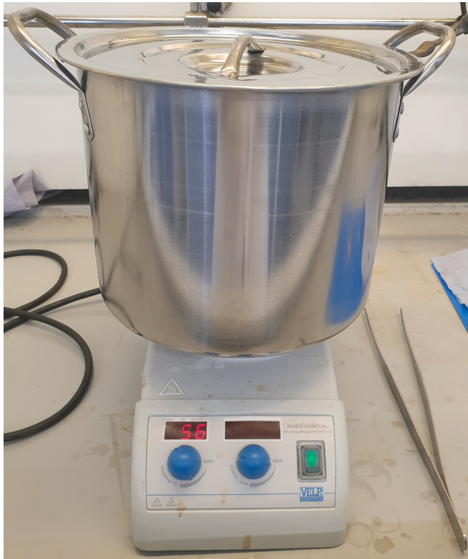
Fig. 2. Stockpot used for washing powder (50°C), and enzymatic maceration (55°C).
