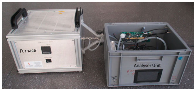
Fig. 6. Photograph of Phi meter furnace and analyser unit.
