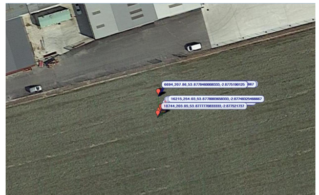
FIGURE 8: Landmine locations with very high MF points filtered from the scanned data in Fig. 7.
