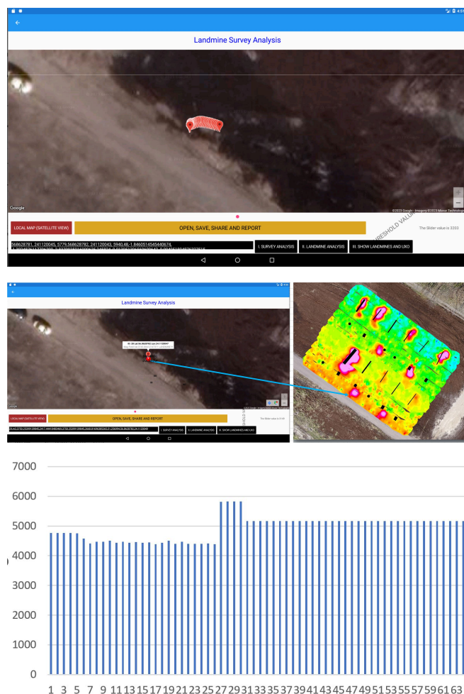
FIGURE 28: Latvia field test -I-. Top: all data points; middle: high MF; bottom: MF graph for all data points in the route depicted at the top. MF is clearly very high at the above location (middle) as shown in the histogram points between 25 and 31.
