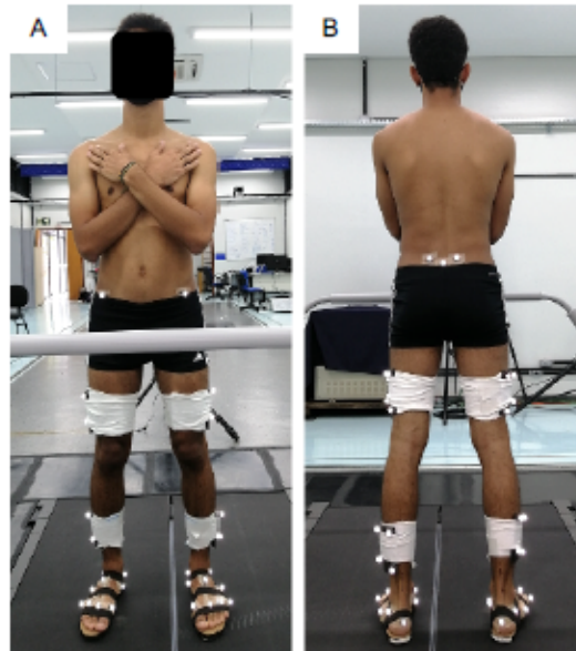
Figure 2: Top: segment definition and marker description. Bottom: anatomical and tracking markers' positions (A and B). Marker type: anatomical (A) and tracking (T).
