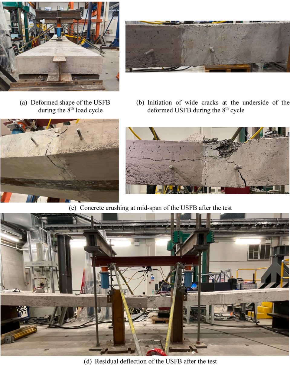
Fig. 10. Failure modes of the composite USFB.
