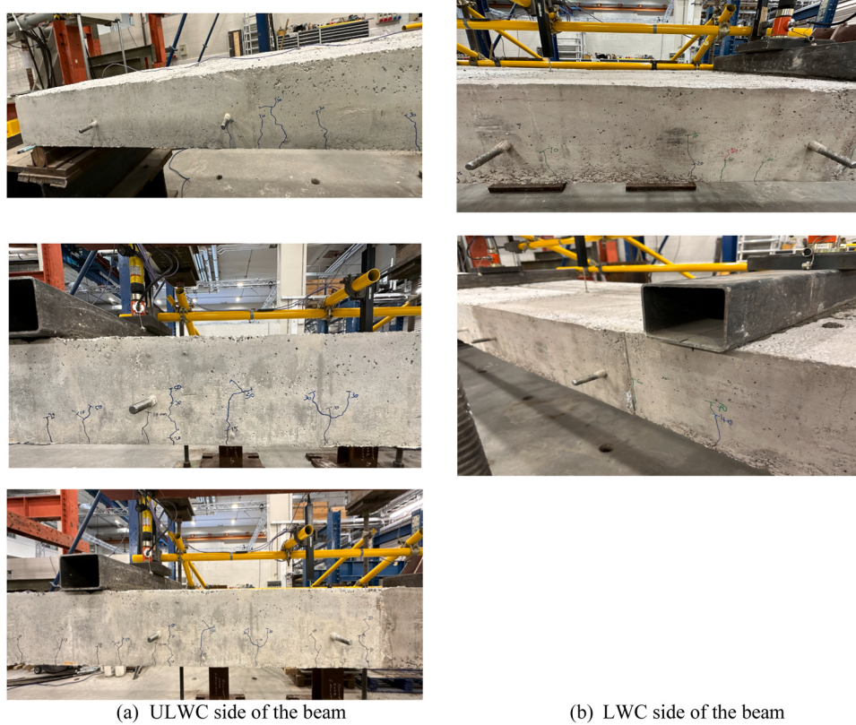
Fig. 11. Concrete crack development.
