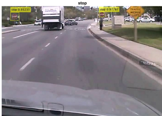
Fig. 7: Faster RCNN detected and drawn bounding boxes with labels around two stop signs.
