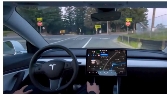
Fig. 8: Still of driverless car video with Faster RCNN traffic sign detector implemented. This frame shows two stop signs are detected with high certainty.
