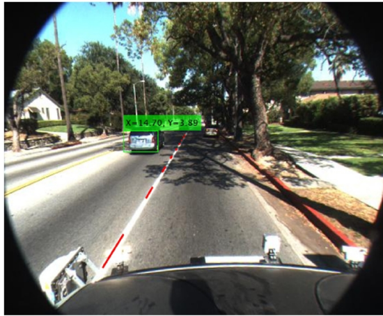
Fig. 10: SSA in Video 1 – instant relative positioning of other vehicles with respect to the ego vehicle.
