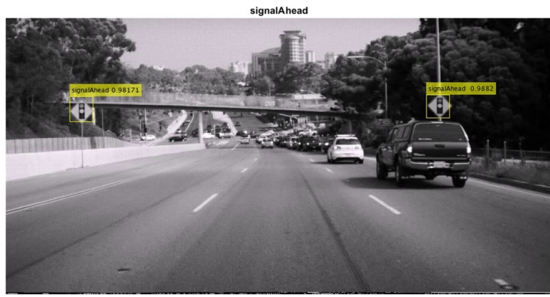
Fig. 6: Faster RCNN detected and drawn bounding boxes with labels around two signal ahead signs.
