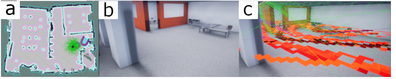
Fig. 1. Preliminary version of the the Digital Twin development process and simulation examples: (a) 2D layout generated through Turtlebot2; (b) 3D Digital Twin; (c) Example ray tracing simulation and heatmap visualisation
