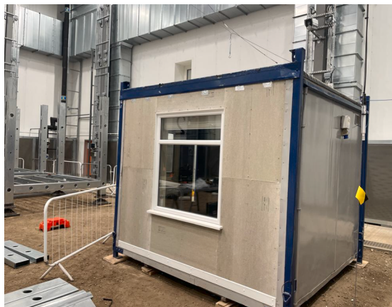
The side view of the completed Thermocill cabin at Salford Energy House (Mar 2023) with full instrumentation
