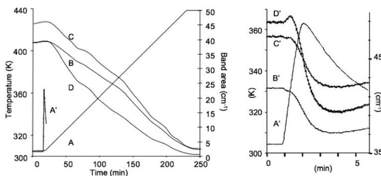
**Fig. 7** Temperature and integrated intensities of water and carbonates bands during conventional (left) and microwave heating (right): A, A'—temperature; B, B'—carbonate band at  $1410\text{ cm}^{-1}$ ; C, C'—water band at  $1635\text{ cm}^{-1}$ ; D, D'—carbonate band at  $1515\text{ cm}^{-1}$ . The temperature increase (A') during the microwave experiment is added in the data for the conventional heating for the sake of comparison.
