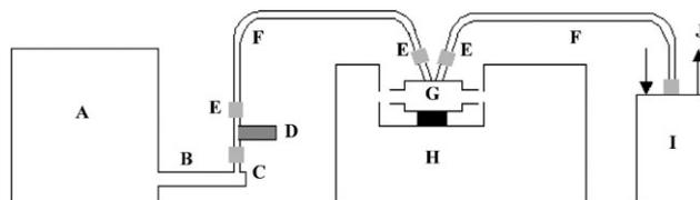
**Fig. 3** Experimental setup: A—microwave generator; B—waveguide; C—waveguide-coaxial transition; D—coaxial sliding short; E—coaxial cable connections; F—coaxial cables; G—reactor-cell; H—FTIR spectrometer; I—water load; J—water cooling circulation.
