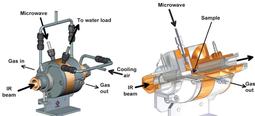
**Fig. 1** General view of the microwave reactor–IR cell.
