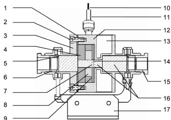
**Fig. 2** Microwave reactor–IR cell (longitudinal cut). 1—TGBS gasket; 2—cell closing screw; 3—stainless steel lid; 4—Macor<sup>®</sup> filler; 5—o-ring; 6—stainless steel nut; 7,8—microwave active brass grid and body of applicator; 9—Macor<sup>®</sup> sample holder; 10—copper wire; 11—1/4" pipe; 12—brass body; 13—heating element; 14—sample; 15—brass nut; 16 KBr and CaF<sub>2</sub> windows; 17—cell stand.
