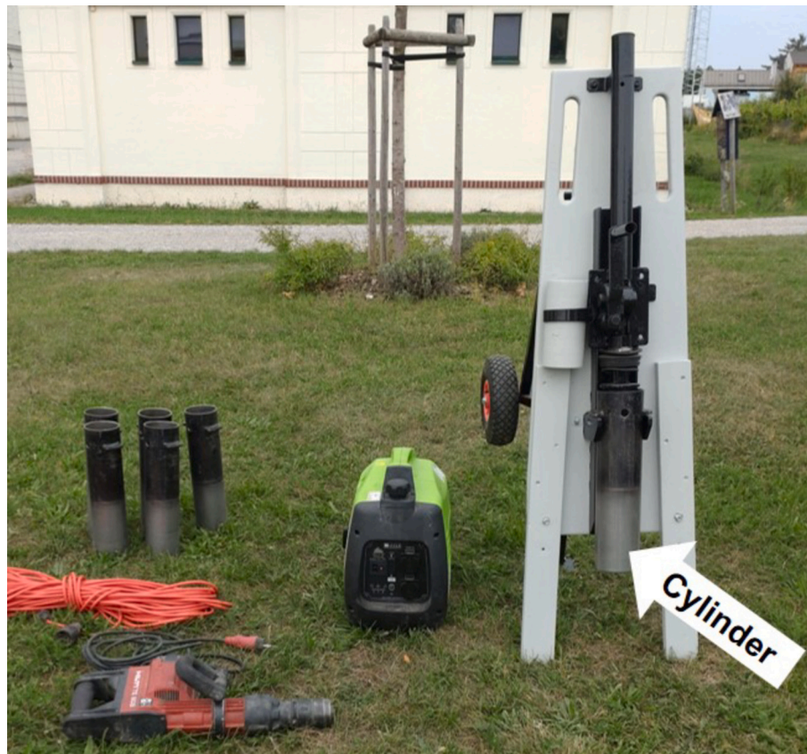
Fig. 1. Cylinder extractor with six cylinders (10 cm diameter, 50 cm length), power generator, electric cable and electric heavy-duty demolition hammer.
