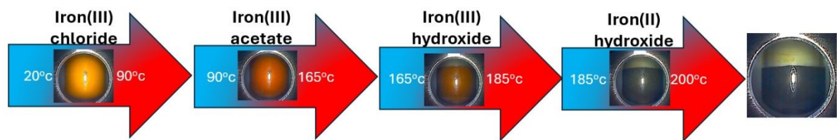
Fig 2 Image of reaction mixture during microwave synthesis demonstrating the different states present depending on reaction temperature transition. The time lapse in any temperature range depending on ramp rate will impact the nature and predominance of the species present.
