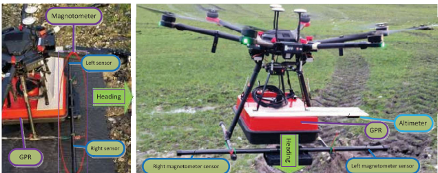
FIGURE 5. Onboard sensors: Magnetometer and GPR.
