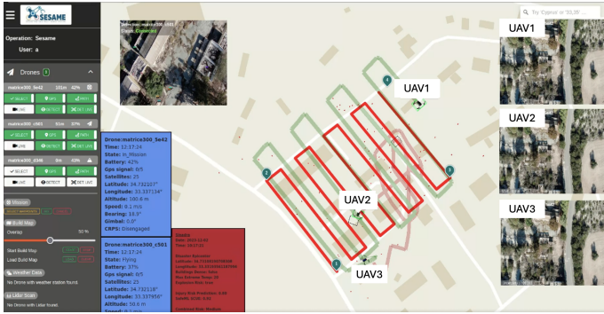
Fig. 4. SESAME multi-UAV platform with the three UAVs operating the SAR algorithm and the integration of SESAME EDDI technologies
