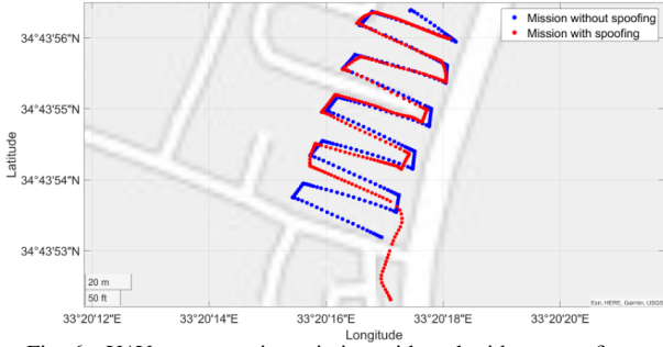
Fig. 6. UAV area mapping mission with and without spoofing attack
