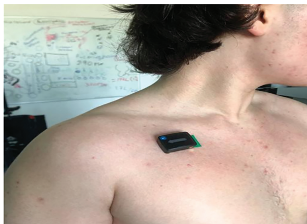
Fig. 1. Delsys EMG sensor set on the clavicular head of the PM muscle.
