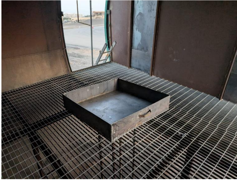
Figure 93: Fuel pan height located 0.3 m from the floor.
