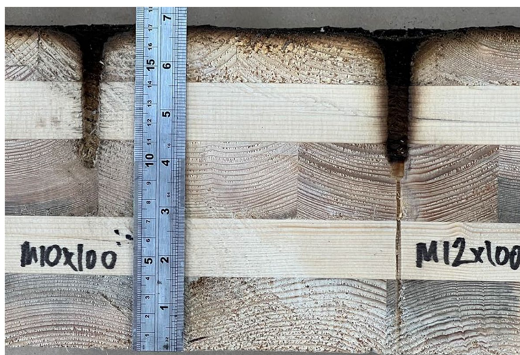
Fig. 15 Enlarged view of internal charring through heat conduction at the coach screws
