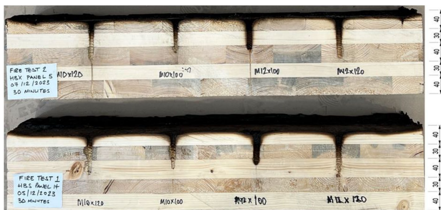
Fig. 13 Cross section of tests FT1 and FT2 showing loss of material at the surface of the CLT panel and the 'dishing' effect localised around the screw fixings after 30 min fire exposure
