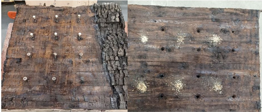
Fig. 11 CLT panel with the char removed around the screw fixings (left) and pilot drill holes for remaining slab thickness measurements (right)
