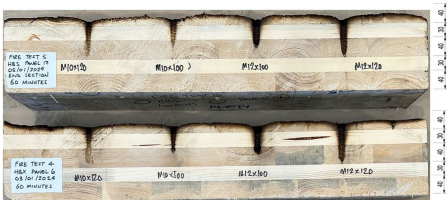
Fig. 14 Cross section of tests FT4 and FT5 showing loss of material at the surface of the CLT panel and the ‘dishing’ effect localised around the screw fixings after 60 min fire exposure
