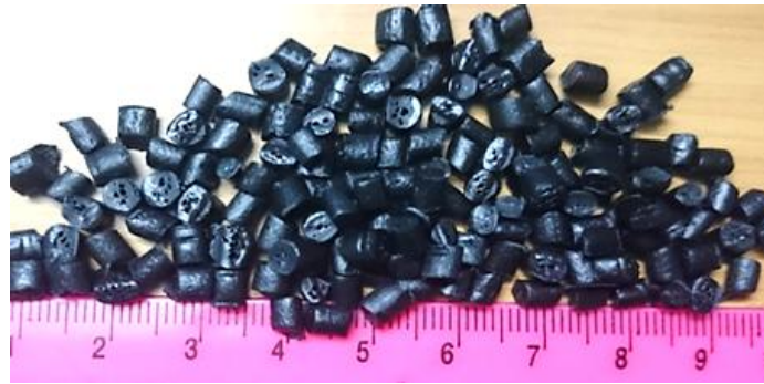
Figure 1. Polycarbonate (PC) plastic waste aggregates used in this study
