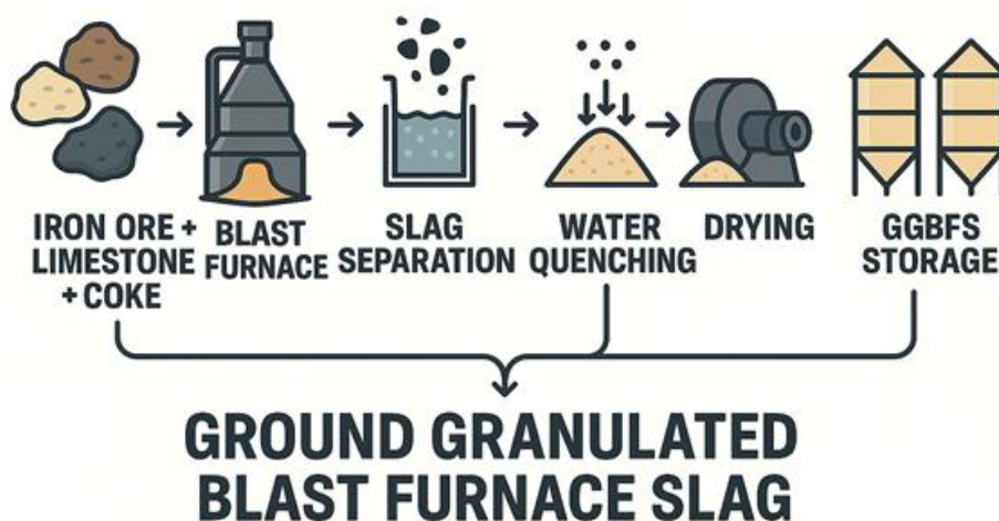
Fig. 3: Schematic representation of the GGBFS production process.
