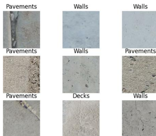
Figure 2. Sample annotated images from the dataset used for crack detection.
