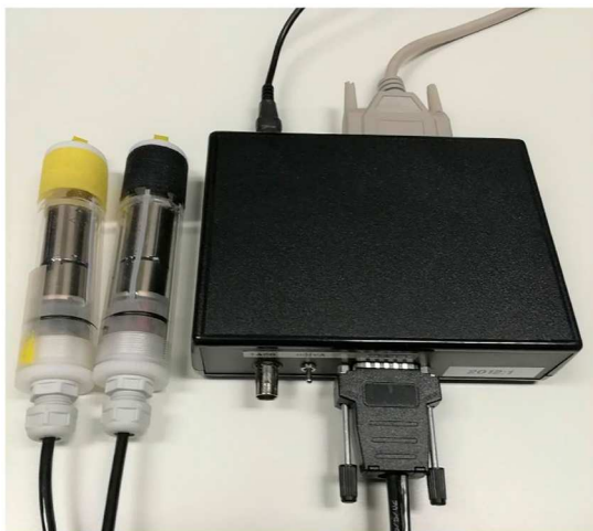
Figure 1. A picture of the vibrotactile stimulation device. Handles that would deliver vibrations are shown to the left, and to the right of them is the control unit. Participants would hold the handles during the stimulus phase of the serial recall task.
