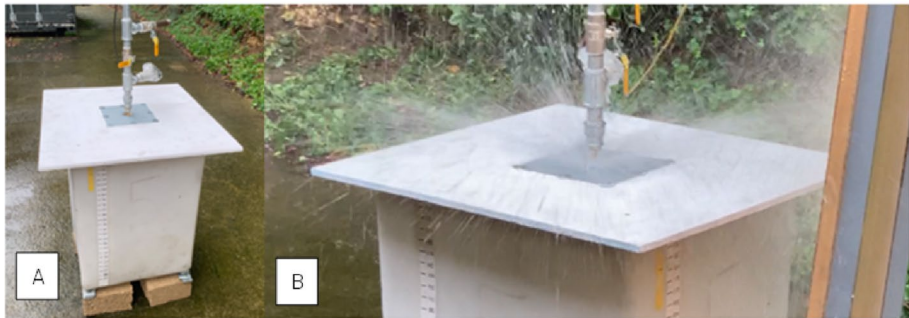
Fig. 4 Simplified test set-up for recording below water distribution capture from sprinklers. A The test set-up. B Water capture below the sprinkler
