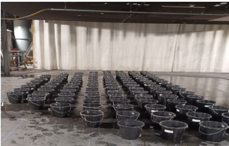
Fig. 8 Water collection buckets in a semi-circular layout below the sprinkler
