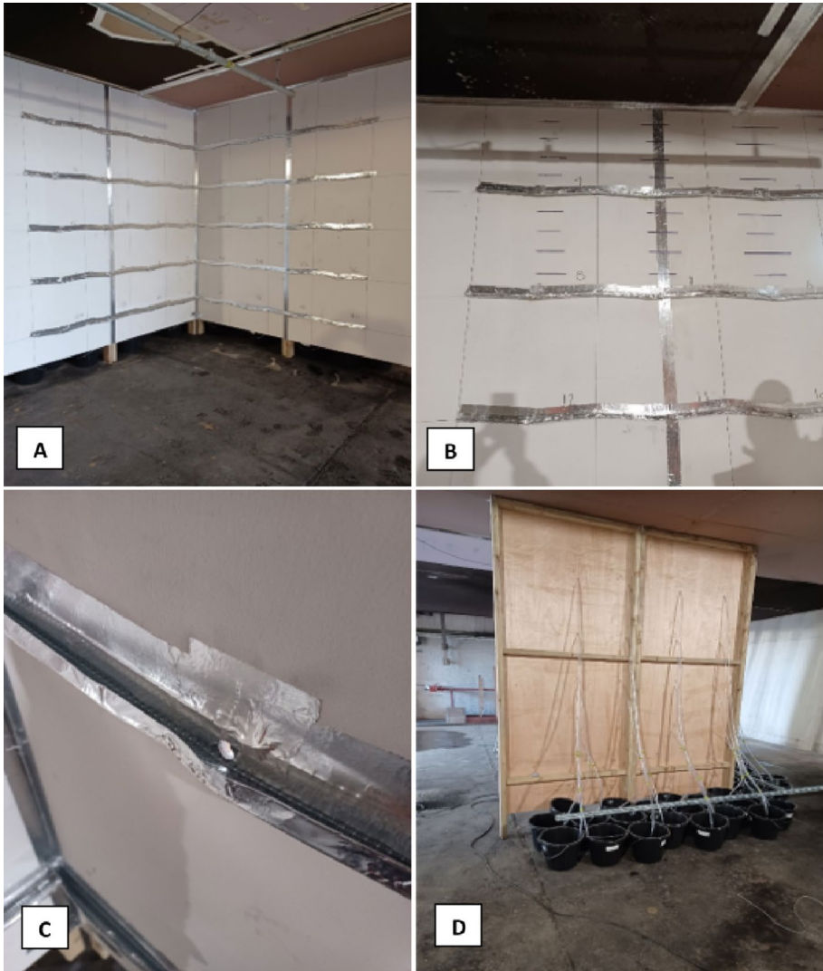
Fig. 18 a Corner wall set-up. b 0.5 \times 0.5 m ( 0.25 \text{ m}^2 ) measured area. c Water collection trough. d Water collection buckets with clear tube feed pipes at the rear
