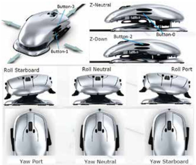
Fig. 4. Essential attributes: The mapping of the WING to the rotational orientations with three degrees – roll ( \phi ), pitch ( \theta ) and yaw ( \psi ) channels
