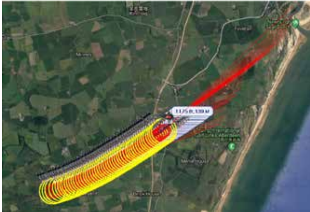
Fig. 9. Generation of future waypoints: safety travel tube with estimationbased predictive display
