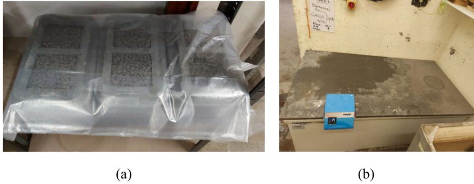
Figure 8. Curing of specimens: (a) initial curing (b) final curing by water immersion.
