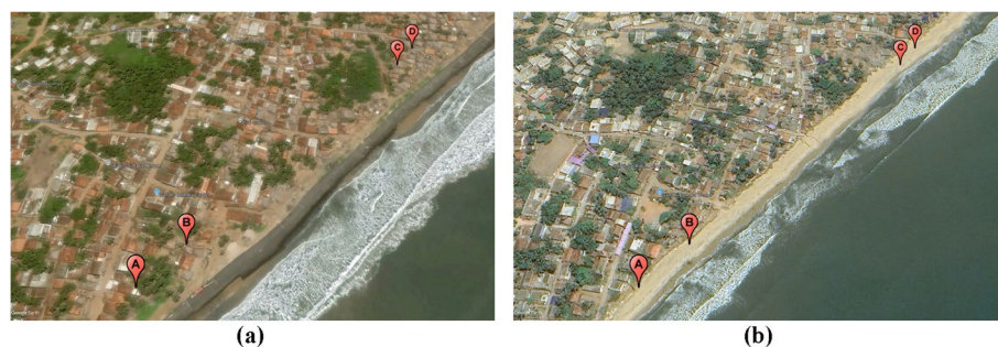
Fig. 20 Comparison of coastal erosion at identified locations (A, B, C, and D) during the field visit, using Google Earth images from 2011 to 2024. The marked locations, which were inland in 2011 (a), had shifted to the shoreline by 2024 (b), highlighting significant erosion over time. Source: Created by the second author using Google Earth Pro 7.3.6
